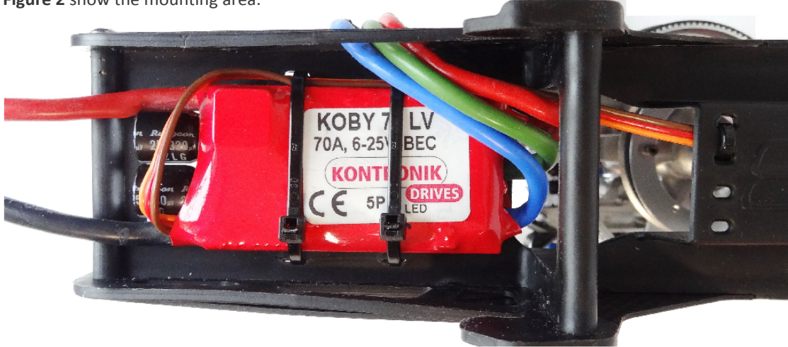
Figure 3: Shows the correct use of the Zip-Ties
