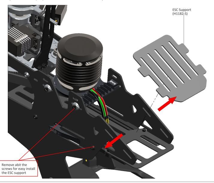
Figure Shows the ESC installed.
