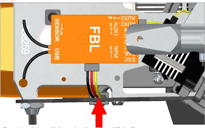
The area between the boom and the frame can be used to route the wire(s) (Fig 4 and 5).
